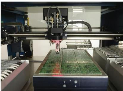
Semi-conductor pick and place robotics
