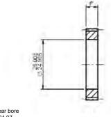
Delrin gear bore Ø25.02/24.97
