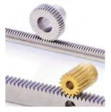
The racks are manufactured from ground, hardened stainless steel or ground stainless steel and available with a choice of accuracies, pitches, and lengths, plus the facility to provide modifications such as flats, journals or custom ends. Hobbed stainless steel and brass racks are also available. The rack pinions are plain or anti-backlash, also with a choice of accuracies, pitches, bore sizes, alternative materials and coatings.
