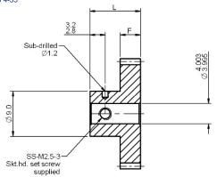
All dimensions in mm General tolerances ±0.13 mm Pressure angle 20°
