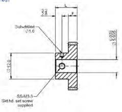
All dimensions in mm General tolerances ±0.13 mm Material: Stainless steel 17-4 PH, hardened to 35-42 HRc Pressure angle 20°
