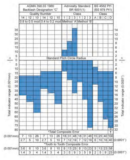
\*AGMA values quoted are for over 20T up to 50 mm (2") diameter. Admiralty and B.S. tooth to tooth errors are for over 30T.
