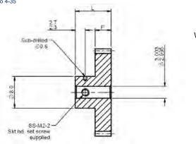
All dimensions in mm General tolerances ±0.13 mm Pressure angle 20°
