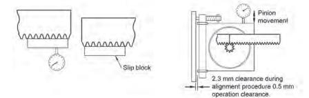
The flexplate spring loads the pinion into mesh on both flanks of the teeth, ensuring complete backlash elimination.
