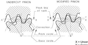
X = Uncorrected PCD Y = Corrected PCD
