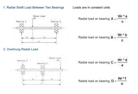
The individual bearing loads can then be used to predict the bearing life.
