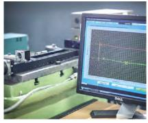
Gearbox Transmission Error Measurement (TEMS) trace
