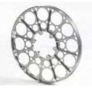
During manufacturing all gears are individually inspected for gear quality and size using a dual flank inspection process with maximum accuracies of 3 microns tooth-totooth and 5 microns total composite error. For demanding applications gears are inspected for lead, pitch and profile on our Klingelnberg P40 gear measuring machine.
