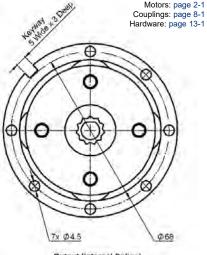
Output (Internal Spline) Splined hole Ø12 11 Splines 1 Module, 45" P A
