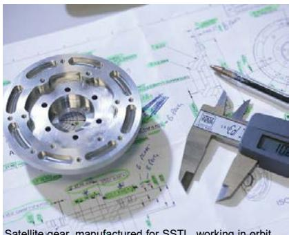
Satellite gear, manufactured for SSTL, working in orbit
