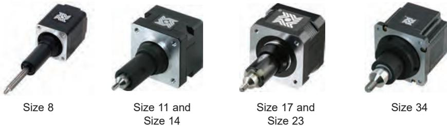
External linear actuators combine conventional leadscrew and nut technology with stepper motor technology. The leadscrew forms part of the motor shaft negating the need for a shaft to shaft coupling, thus providing zero transmission error from motor to screw and shortening the overall linear footprint.
