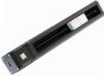
The carriage design is unique; it controls slide bearing play with a self-adjusting linear bearing. Integrated along the entire length rail system are “T” slots allowing mounting of limit switches and sensors.
