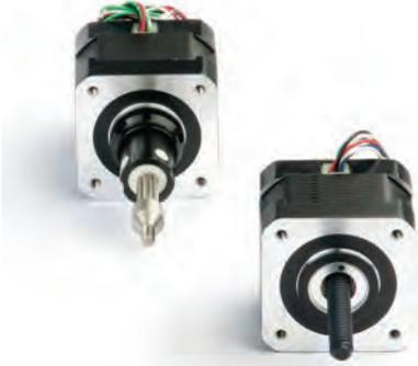
The hybrid linear actuators are available in NEMA frame sizes 8 to 34, with up to 400 full steps per revolution and travel increments as small as 0.003 mm/step.
