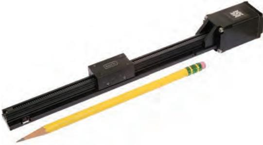
The motorised leadscrew linear slide features wear-compensating, anti-backlash carriages to ensure repeatable and accurate positioning. The pre-assembled unit combines a screw-driven linear actuator with an integrated stepper motor drive reducing part count and improving system integration.
