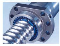
Combination wipers are plastic wipers with an additional felt wiper (inside the ball nut). They are used where felt wipers are desirable, but need to be protected from water or water based fluids. Felt tends to absorb water, so it should not be used without the additional plastic wiper in such cases.
