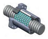
Steinmeyer's "UltraSpeed" return is normally used for lead/diameter ratios greater than 0.5. It is normally used with dual start threads. Balls are lifted off the shaft using a deflector at one end of the nut and then guided through a bore (internal to the nut body) to the other end of the nut, where a similar piece guides the balls back onto the thread. One pair of deflectors serves one circuit (i.e. one of the threads) which includes several turns.
