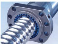
Plastic wipers, sometimes called "labyrinth seals", are widely used in machine applications. They prevent contamination of the nut from chips and other larger particles, while at the same time letting some oil exit the nut. Combined with automatic grease or oil lubrication, they help to flush the nut. The result is higher reliability of the ball screw.
