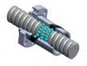
The track-to-track return uses ball deflectors to lift the balls across the O.D. of the shaft and guide them directly into the next (or previous) track. Internal ball return is very compact and yields the smallest nut diameters among all ball return systems. It is also the ball return of choice for very small ball sizes and small leads.
