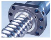
Felt wipers are an excellent solution for ball screws operated in an environment with abrasive or otherwise troublesome dirt as in grinding or woodworking machines (for example oil absorbing particles like wood chips). The felt wiper seals the nut effectively, even from fine particles, and also stores some lubricant. Felt wipers are contact wipers and add some friction.
