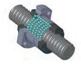
End cap return works very much like the previously described through-the-nut return, with the exception that the ball deflector function is executed using a (plastic) cap at both ends of the ball nut. Each cap serves as the ball return and also includes wipers. End cap return is normally used for very large lead/diameter ratios. This style ball nut is only available as a flange nut.
