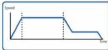
**Push Mode:** Mimics a typical pneumatic motion. It keeps pushing for a given time and at a set current level when a motor encounters a resistance such as a bumper or stopper.
