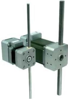
Multiple configurations are available developing peak forces up to 150 N and rated speeds of 300 mm per second, with resolutions of better than 1 micron and standby power consumption of less than 1.7 watts. The assembly has a number of different mounting options for ease of mechanical installation.
