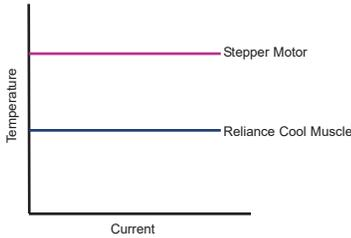
RCM applies optimum current to produce motion, whereas an open loop stepper always uses maximum current.
