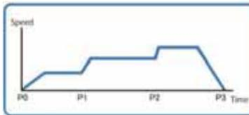
**Continuous PTP:** There are no stops in motion between origin and P3. Speed and acceleration are changed at each point.
